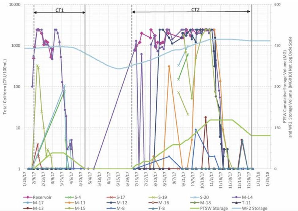
Figure 4. Partially Treated Surface Water Cycle Testing – Total Coliform
