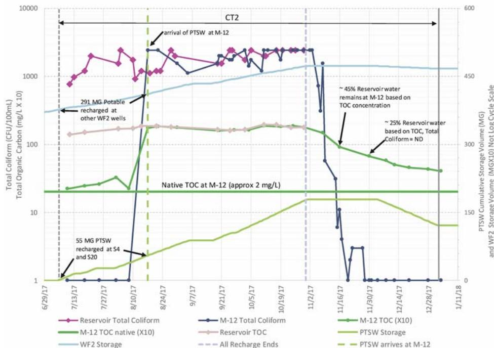
Figure 5. Partially Treated Surface Water Cycle Testing – M-12 Total Coliform and Total Organic Carbon
